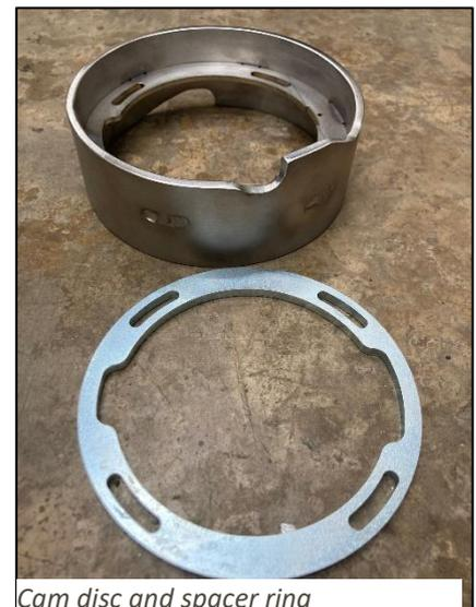
*Cam disc and spacer ring*
