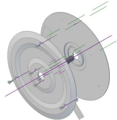
**To remove the blades, simply loosen the corresponding screw that holds the blade with spacer ring.** Proceed as follows:
