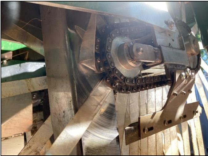
*Blockage due to stuck slat*
