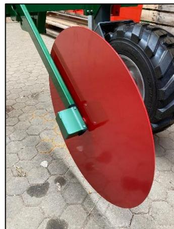
*Protective disc with speed sensor*
