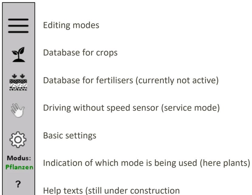
The fertiliser database is only active if MulchTec fertiliser boxes are part of the machine equipment.
