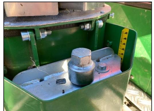
*Height adjustment of the pressure wheels using a 24 mm hexagon and tilting of the wheels in relation to each other using*
